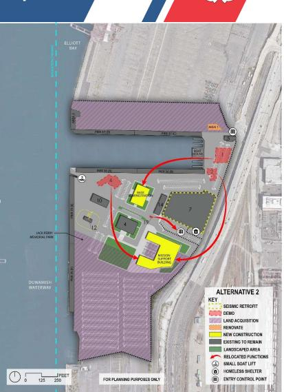
**Base Security and Fencing:** Replace Main Gate with Anti-Terrorism/Force Protection (AT/FP)-compliant main entry control point (ECP), replace secondary gate with AT/FP-compliant ancillary ECP, and install security barriers and pavement, overhead security lighting, Main Gate Security Gatehouse, and security sensors.
